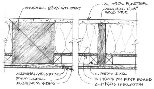
Condition: Although it is difficult to assess the condition of the outside of the exterior walls due to the presence of aluminum siding, they appear to be generally sound and in good condition. Some potential areas of deterioration were identified at the exterior where roof water management and flashing are inadequate, however the exact conditions of these concealed areas are not known. However they are not believed to be serious, and may be limited to localized wood siding deterioration.
